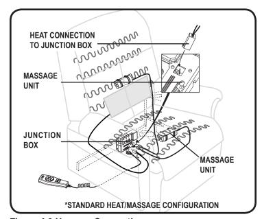
**Figure 4.2 Harness Connections**
