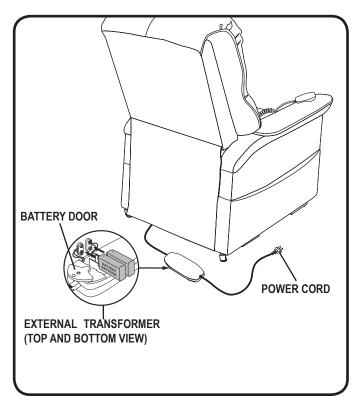
Figure 4.3 Chair Battery Back-up Location
