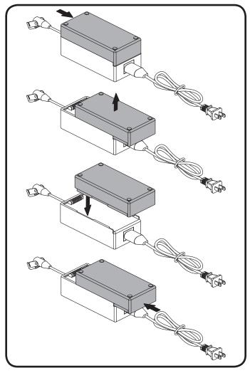
Figure 4.5 Lithium-Ion Battery Replacement
