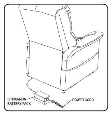
Figure 4.4 Chair Battery Back-up Location
