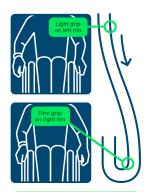
To turn while the motor is driving, grip either handrim firmly to make a sharp turn or to turn around completely.
