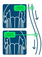
To steer while the motor is driving, lightly grip either handrim to turn in the direction you would like to go.
