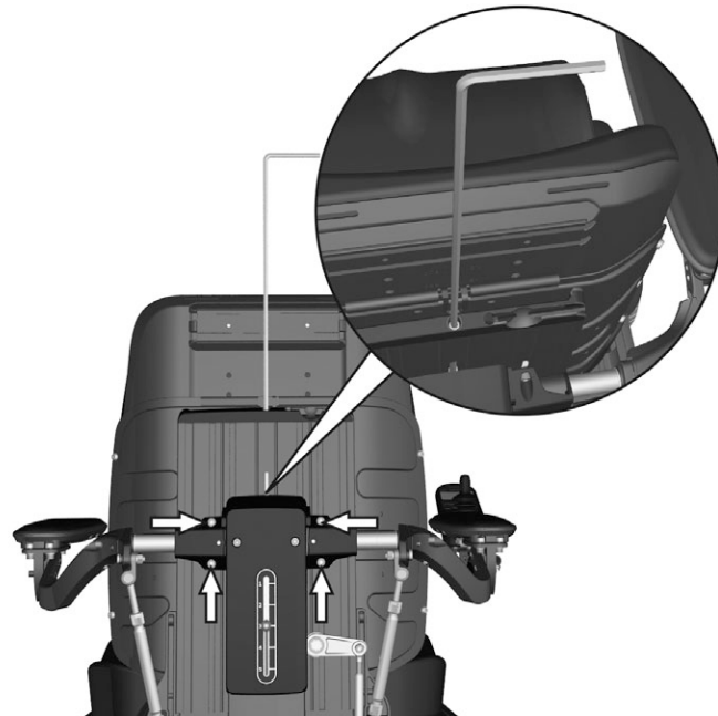
Figure 22. Adjusting the arm rest height
