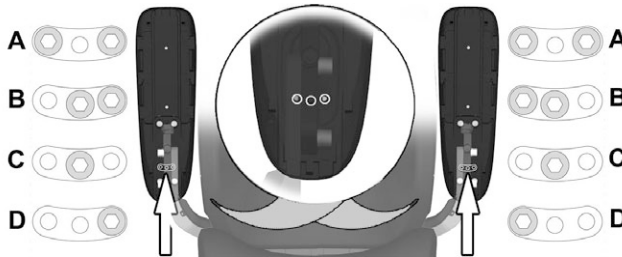
Figure 21. The endpoints are set by moving one or two screws between three different positions underneath the arm rest.
