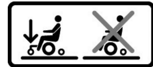
Figure 123. The support wheels must always be fitted when you drive.
