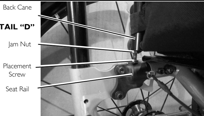
FIGURE 2 Back Angle Adjustment
