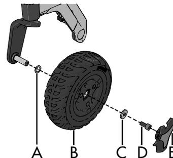
Figure 166. Assembly of rim.
