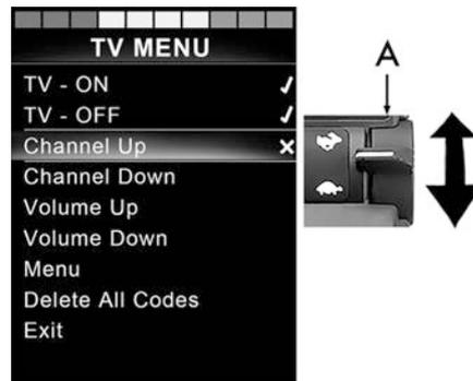
Figure 92. Screen and speed paddle switch marked A.
