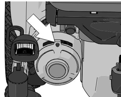
Figure 136. Release lever location.
