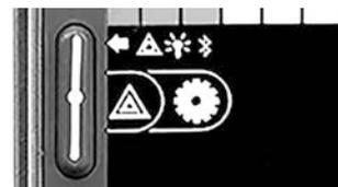
Figure 75. Button to access settings in Bluetooth® mode.
