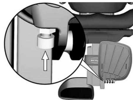
Figure 22. Footplate angle stop screw.
