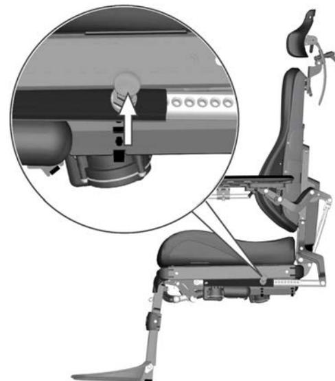
Figure 18. Manually adjusting backrest angle.
