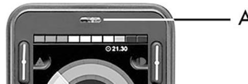
Figure 83. The IR receiver location.
