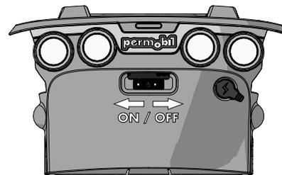
Figure 8. Main circuit breaker location.
