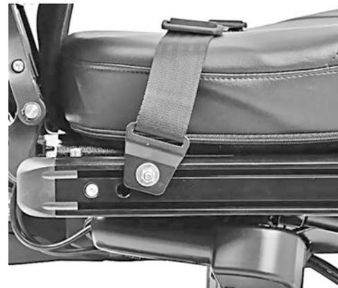
Figure 35. Attaching the positioning belt.
