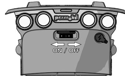
Figure 192. Main circuit breaker located under the rear lights.
