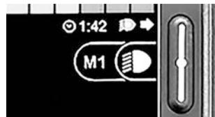
Figure 76. Button to return to drive mode from Bluetooth® mode.
