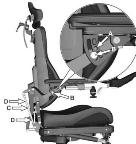
Figure 27. Adjusting the armrest height and angle.
