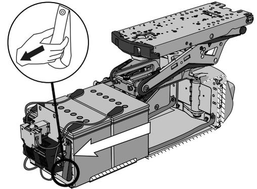
Figure 179. Straps for pulling out battery box.
