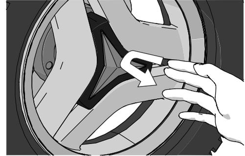
Figure 154. Use your fingers as follows on two edges of the hub cap.
