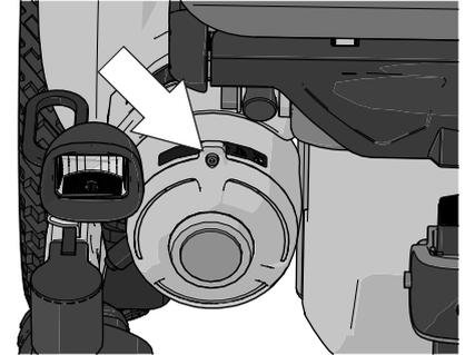
Figure 148. Brake release lever.
