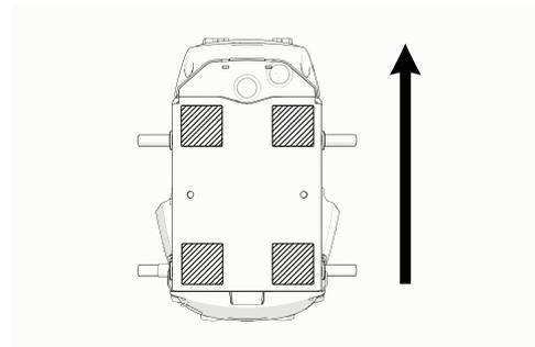
Figure 165. The position of the blocks. The arrow points in the direction of travel.
