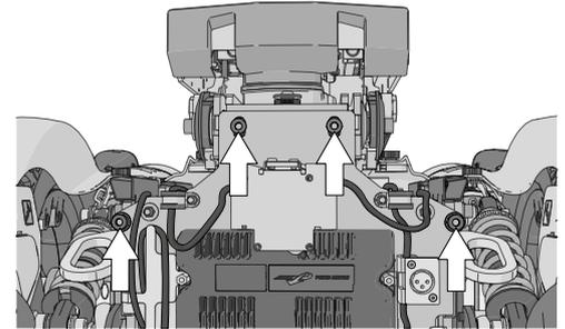
Figure 187. The battery box is secured with four bolts.
