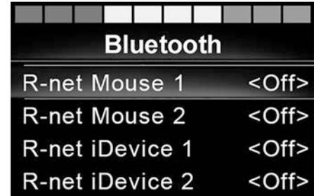
Figure 69. The Bluetooth® submenu.
