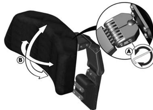
Figure 42. Adjustment of headrest angle.
