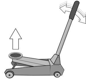
Figure 163. Use a jack or equivalent to lift up the wheelchair.
