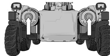
Figure 5. Front reflectors.
