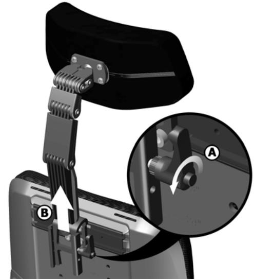
Figure 39. Removal of headrest.
