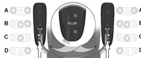
Figure 24. Adjusting the armrest swivel end position.
