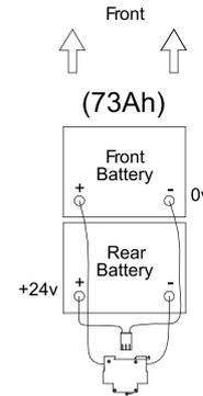
Figure 182. Wiring diagram for the batteries.
