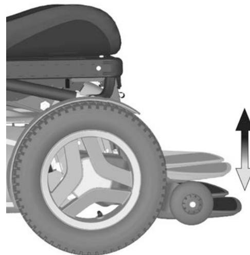
Figure 1.5. Power adjustable leg length.
