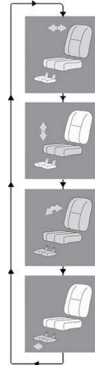
Figure 97. Move the joystick to the left or right to select a function. The icon for the seat function selected appears in the display.
