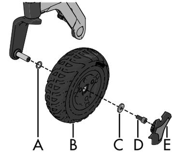
Figure 167. Assembly of rim.
