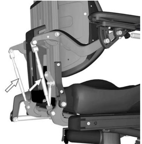
Figure 26. Armrest angle adjustment bars.
