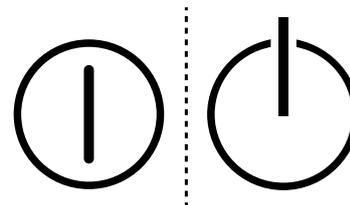
Figure 150. On/Off symbol depending on model.
