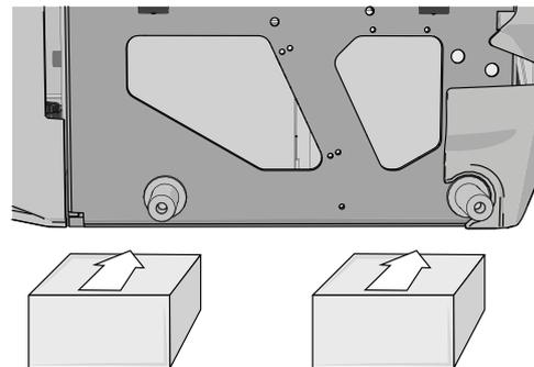
Figure 152. Use two blocks on each side of the chassis box. The wheels has been removed in this figure for better viewing.
