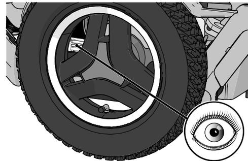
Figure 144. Chassis identification number label.
