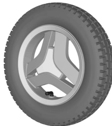
Figure 160. Filling valve on drive wheel.
