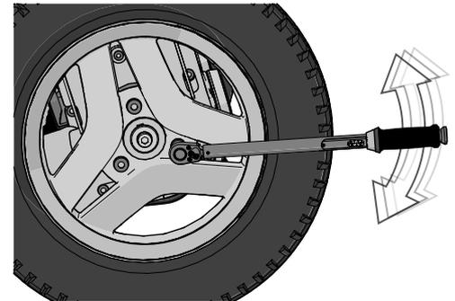
Figure 157. Use a torque wrench to tighten the screws.
