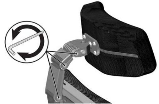
Figure 41. Adjust height and depth.
