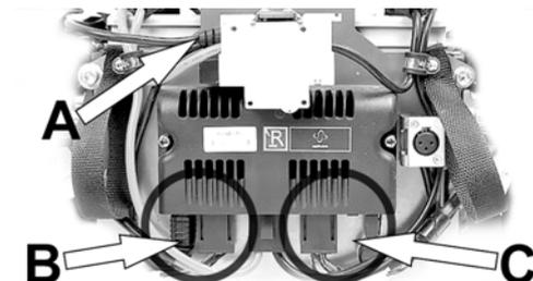
Figure 178. Connectors (B) and (C); for disconnection.
