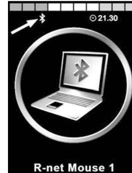
Figure 70. The arrow points to the flashing Bluetooth® icon.
