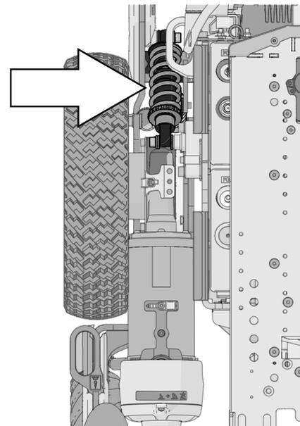
Figure 4. Drive unit and shock absorber.
