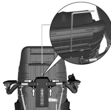
Figure 25. Adjusting the armrest height.
