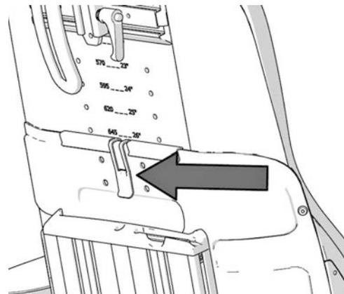
Figure 28. Clip holding the backrest.
