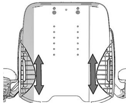
Figure 31. Adjusting trunk support height.
