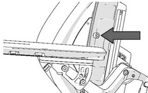
Figure 30. Trunk support screw.
