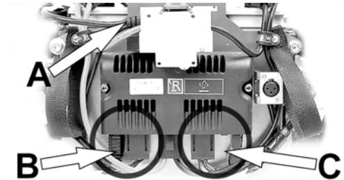
Figure 186. Connectors (B) and (C); for connection.
