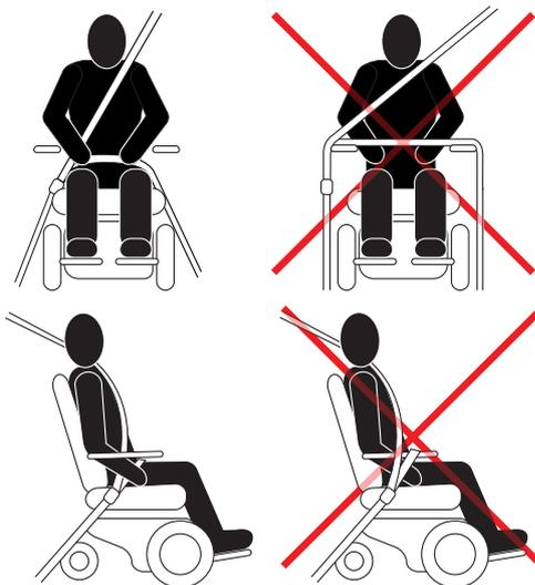
Figure 143. The left figures show the correct positioning of the seat belt.
