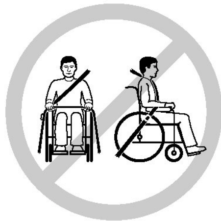
Incorrect seat belt position
