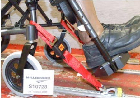
Fitting the front restraint
