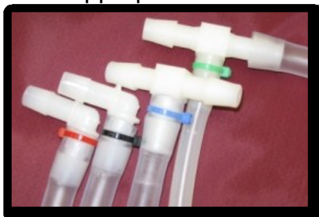
Figure 16: Color-Coding of CPR Hoses Inside Mattress
