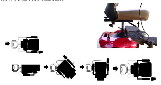
Above: Seat shown in the four possible "ENGAGED" positions Below: Seat shown in the four possible "REMOVABLE" positions
