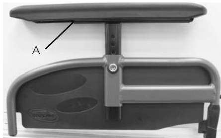
FIGURE 6 Replacing Armrest Arm Pad
