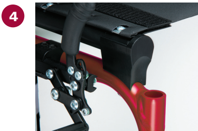
4 A front capped H-block helps rigidize the frame by holding the seat rails in place.
