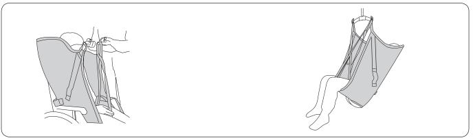
**Tip:** Check that all suspension loops have the same length, i.e., are at an equal height when they are stretched prior to lifting. Adjust the position of the sling if they are not at an equal height.
