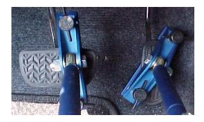
3. You should be able to slide the brake mount over the pedal in a vertical placement. Then tighten finger screws evenly and verify that the clamps are secure. Be sure that the AZ-1 portable hand control system doesn't interfere with anything that would compromise safety. If the AZ-1 cannot be adjusted to the proper length contact the company where you purchased and return for replacement immediately.
