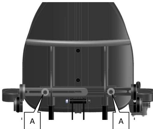
Untighten the two screws (A), now you can slide the armrests stepless in the width.
