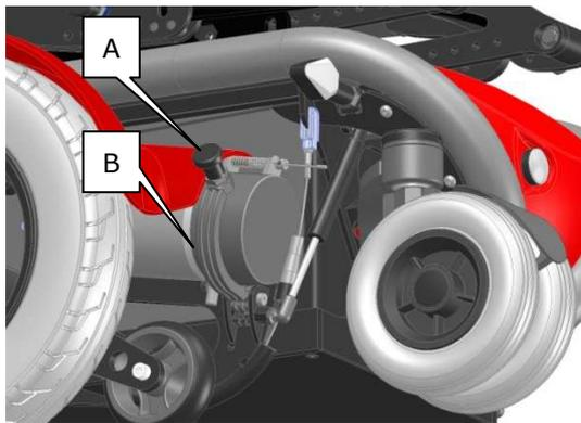
To disengage the motor brakes, to push the chair manually, switch off the control, pull the quick release knob (A) and press the lever (B) down.
