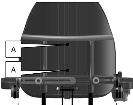
You can adjust the height of the backrest by untighten the two screws (A) a bit. Then you're able to shift the backrest up and down. If the backrest is in the desired position, tighten the screws (A).
