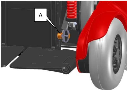
To change the height of the footrest, pull out the quick release bolt (A), position the footrest at the desired height and put the quick release bolt back in place. There are 4 holes (B) you can use to adjust the height.
