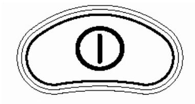
With the On-/ Off-button the chair can be turned on or switched off. Don't use this button to stop the wheelchair, unless there is an emergency.
