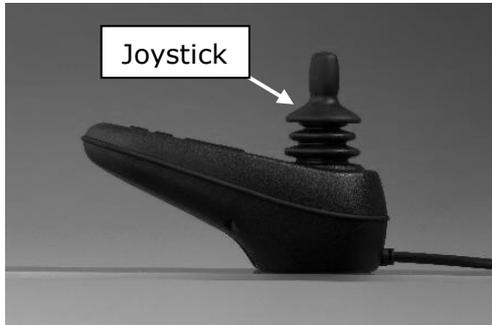
The joystick controls the direction and speed of the wheelchair.
