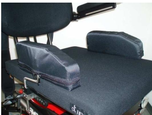
Leads the thigh and stabilizes the leg axle in seating and standing position. Can be adapted individually in place, distance, angle and height. To change the position, open the zipper at the outside of the pad and untighten the screws lightly, now you can adjust the pad to the necessary position, tighten the screws afterwards.
