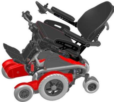
With the option „Tilt in space“ it’s possible to tilt the seat to an angle of 34° to the back, this leads to a more comfortable seat-/ rest-position. The “Tilt in space” is a good prevention against decubitus by the way. In chapter 4.6. you can see how the “Tilt in space” can be adjusted.
