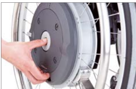
Removing the e-motion wheel from the wheelchair
