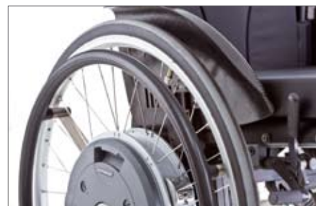
Rubber-coated push rims for improved grip
