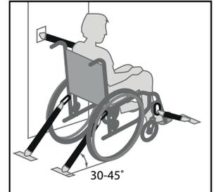
Figure 1. Securing the Wheelchair
